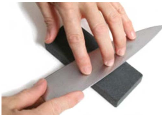
Figure 15 Sharpening the Reverse Side of the Knife
