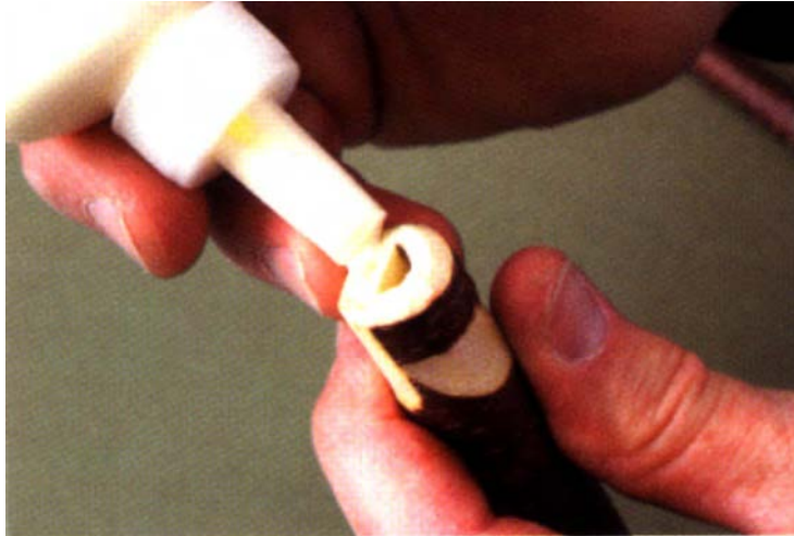
Figure A-11 Glue Cracks
