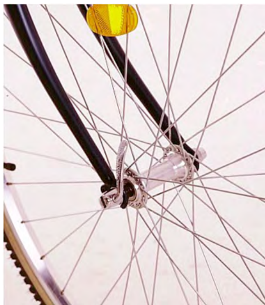
Figure 7 Quick Release Incorrect Position—Example 2
