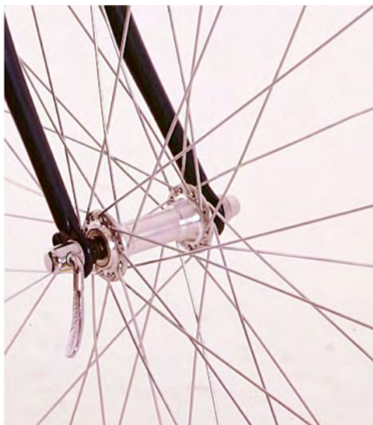
Figure 6 Quick Release Incorrect Position—Example 1
