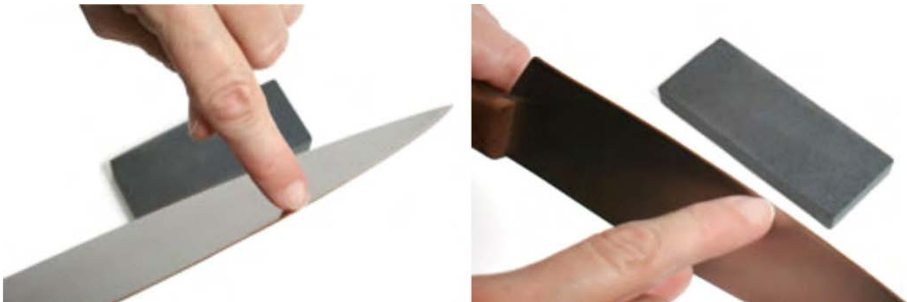
Figure 14 Checking the Bevelled Edge
