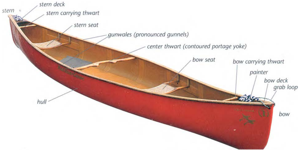
Figure 1 Parts of the Canoe
